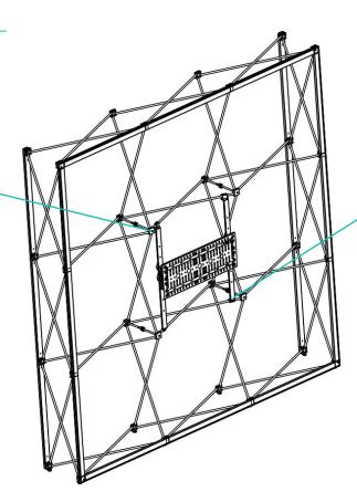
b. Rest bottom brackets on bottom X bars on frame.
